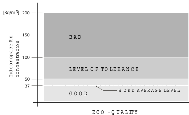
Fig. 3. Determination of the indoor Eco-quality in the function of the Rn concentration.
