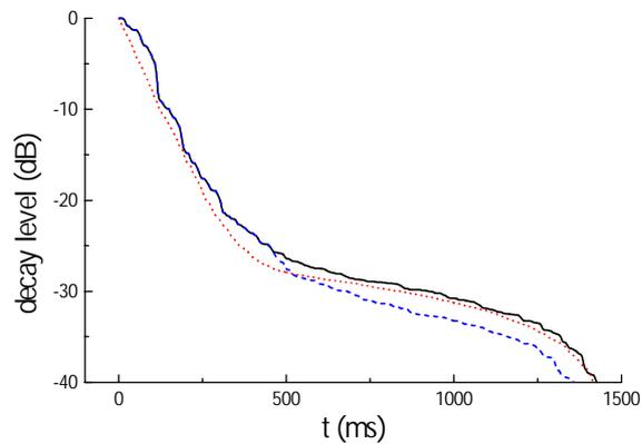
Fig. 4. The decay curves in 1/3 octave band at 200 Hz obtained by pseudorandom noise of order of 17 (—) without equalisation, (- - -) with equalisation and (· · ·) the decay curve at 4 kHz
