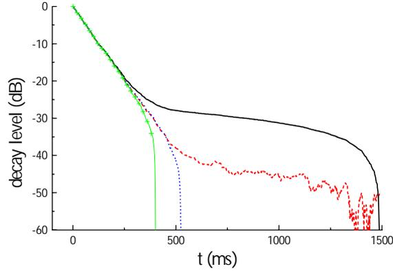
Fig. 7. The decay curves in 1/3 octave band at 4 kHz obtained by pseudorandom noise of order of 17 (—) without the background noise influence reducing, (- - -) by the subtraction of mean square value of background noise and by the impulse response truncation (· · ·) at the knee and (- + -) before the knee
