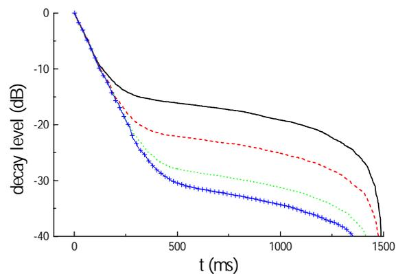
Fig. 5. The decay curves in 1/3 octave band at 4 kHz obtained by pseudorandom noise order of (—) 15, (- - -) 16, (· · ·) 17 and (-+-) 18
