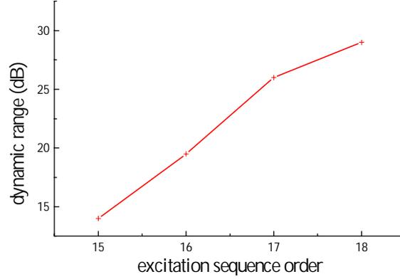
Fig. 6. The averaged results of dynamic range from 100 Hz to 8 kHz versus the pseudorandom noise order
