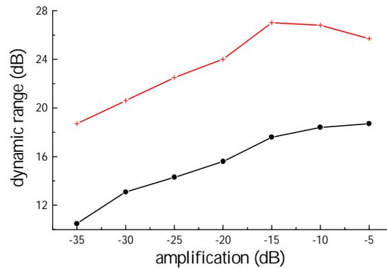
Fig. 3. The averaged results of dynamic range from 100 Hz to 8 kHz obtained by (- + -) pseudorandom noise and (- • -) impulse excitation
