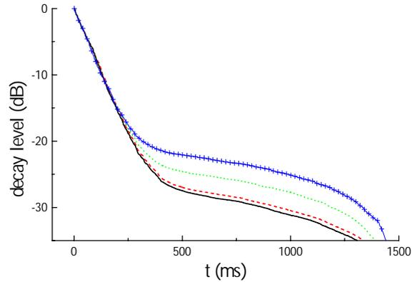
Fig. 2. The decay curves in 1/3 octave band at 4 kHz obtained by pseudorandom noise of order of 17 by using various amplification levels: (- + -) -30 dB, (· · ·) -20 dB, (—) -10 dB and (- - -) -5 dB
