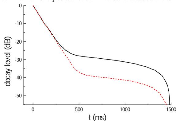
Fig. 8. The decay curves in 1/3 octave band at 4 kHz obtained by pseudorandom noise of order of 17 (—) in one measurement and (- - -) by averaging of results of 10 measurements
