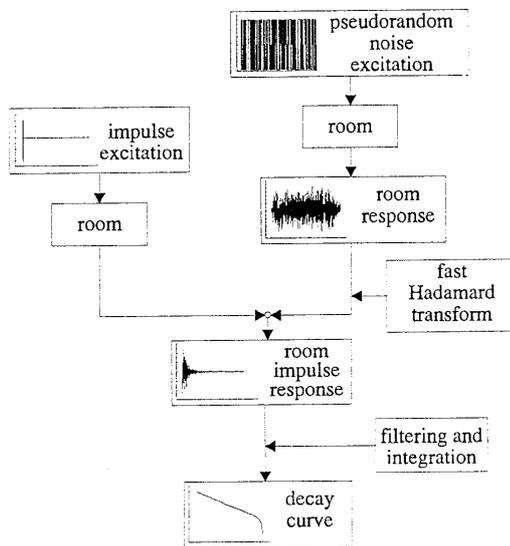
Fig. 1. The measurement procedure
