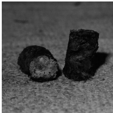
Fig. 1. Heavy biobriquette made of unprepared biomes (grape cuttings)
