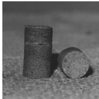
Fig. 2. Heavy biobriquette made of prepared biomes (beech – sawdust)
