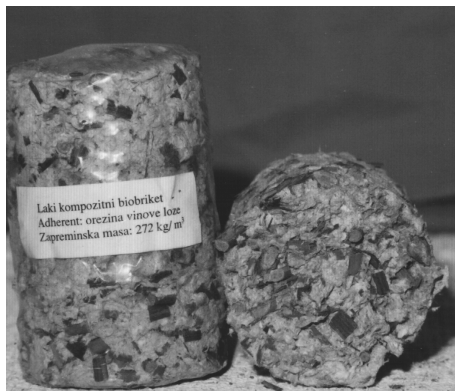
Fig. 3. Light composite biobriquette from grape-vine cuttings and paper pulp as binding mean
