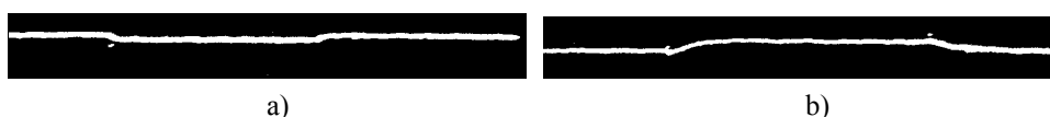
Fig. 1. Electro-optical signal in the solution with c = 0,1 \cdot 10^{-4} \text{ gcm}^{-3} of PAA-A-120 at time duration of rectangular electric pulse t_w = 1 \text{ ms} , temperature T = 25,4^\circ\text{C} and the electric field strength: a) E^2 = 2 \cdot 10^8 \text{ [Vm}^{-1}]^2 ; b) E^2 = 2 \cdot 10^{10} \text{ [Vm}^{-1}]^2
