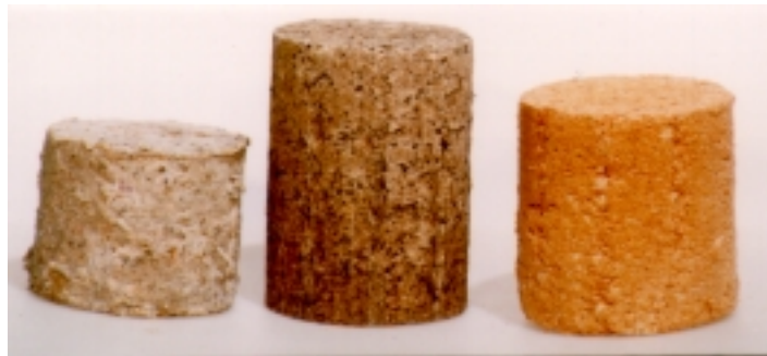
Fig. 2. Light briquette diameter \varnothing 82,5 mm; 1) waste paper pulp (left), 2) paper pulp, coal and limestone (in the middle) and 3) paper pulp and beech sawdust(right); Foto: D. Mitić
