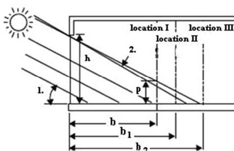
**Fig. 1** A vertical solar window with an ideal thermal mass floor with a width *b*. 1. Solar altitude angle on December 21 at 12<sup>00</sup>, 2. Solar altitude angle on January 21 at 12<sup>00</sup>
