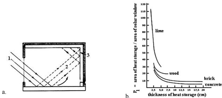
**Fig. 4** a) A cross-section of the room with reflected sunlight radiation, b) The diagram which determined the thickness of heat storage that absorbs the reflected solar radiation: 1. Solar radiation, 2. Reflected solar radiation, 3. Solar radiation reflected by the thermal wall
