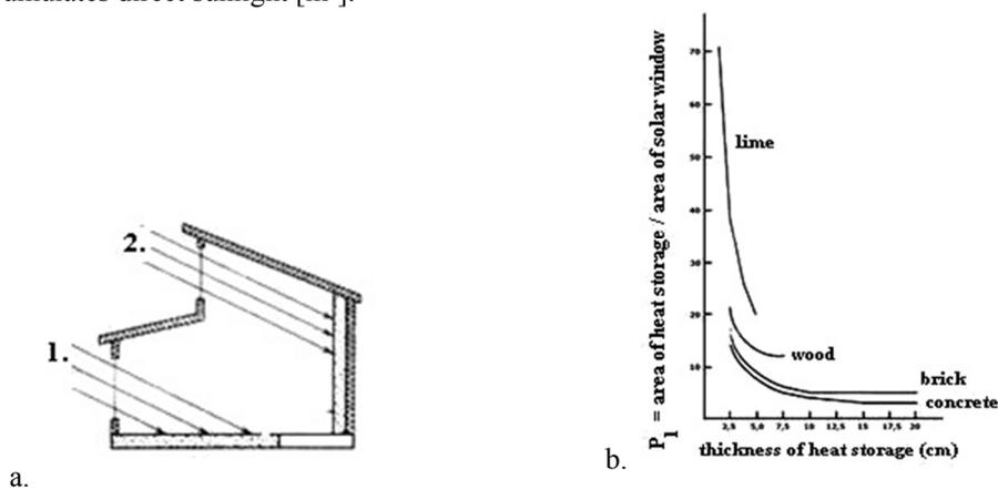
**Fig. 5** a) A cross-section of the room with direct sunlight, b) The diagram with which the thickness of the thermal storage that absorbs direct sunlight can be determined: 1. Direct solar radiation, 2. Direct solar radiation
