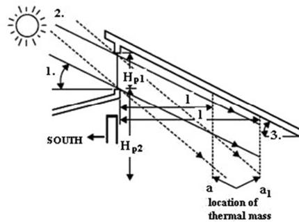
**Fig. 2** Roof solar window: 1. Solar altitude angle on December 21, 2. Solar altitude angle on February 21 and October 21 at 12<sup>00</sup>, 3. Solar altitude angle on December 21 at 12<sup>00</sup>
