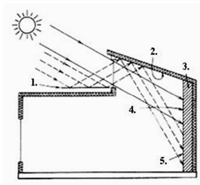
**Fig. 3** Solar skylight with reflective panels: 1. Reflection surface, 2. Internal reflection of solar radiation from the room ceiling, 3. Massive thermal wall, 4. Places of absorbing of reflected solar radiation, 5. Direct solar radiation which is absorbed in the upper part of the thermal wall
