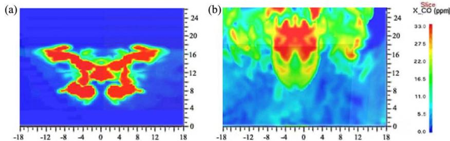
Fig. 6 Leeward (a) and windward (b) fields of carbon monoxide concentrations
