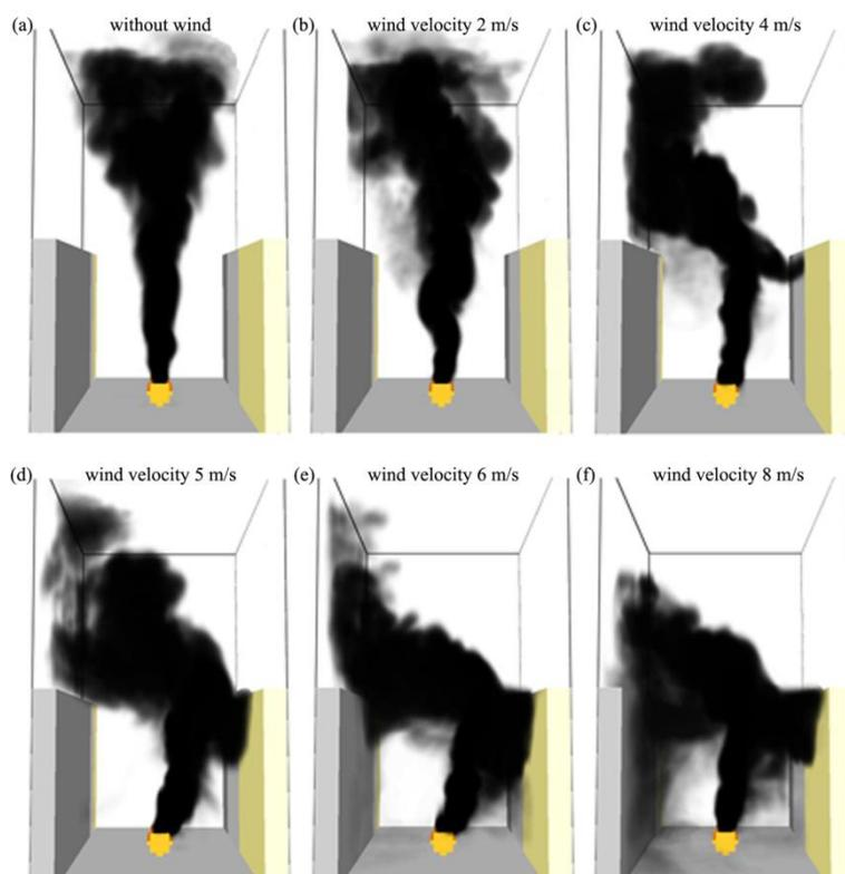
**Fig. 2** The stream of fire products under different wind velocities
