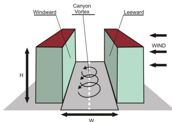
**Fig. 1** The physical model for the LES simulation
