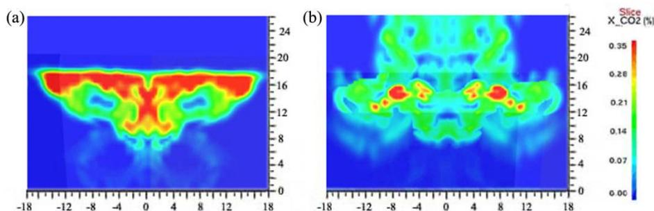
**Fig. 7** Leeward (a) and windward (b) fields of carbon dioxide concentrations
