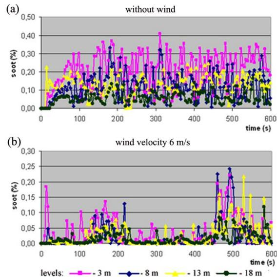
Fig. 5 Soot particles concentrations
