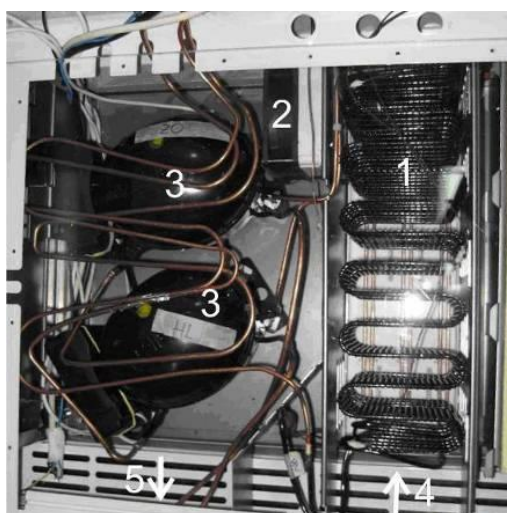
Fig. 1 Elements of a compressor compartment (unit) – basic design: dynamic condenser (1), axial fan (2), two 'variable speed drive' (VSD) compressors (3), air inlet grille (4), air outlet grille (5)
