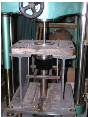
Fig. 1 Experimental pressing stand with heating equipment
