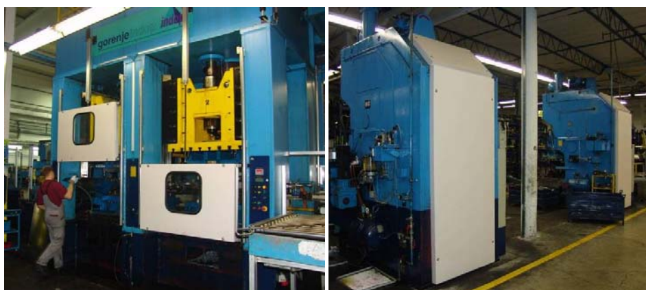
Fig. 5. Acoustic deflectors on the machines.
