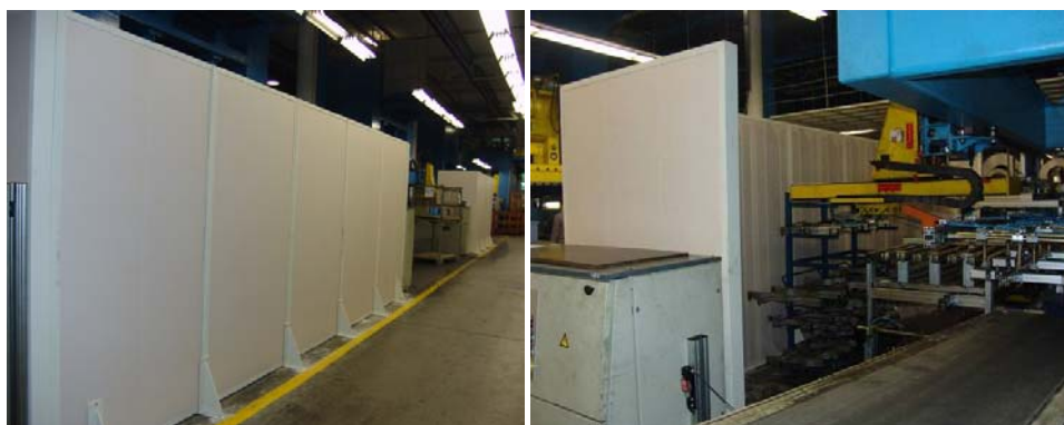
Fig. 4. Sound absorbing barriers on the floor between individual machines.
