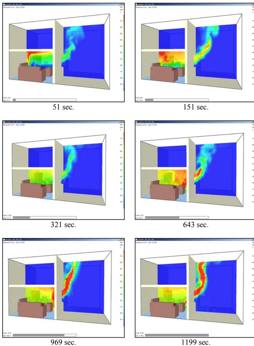
**Fig. 3** Temperature Schedule at Axes Opening from 51 to 1199 Seconds since Ignition
