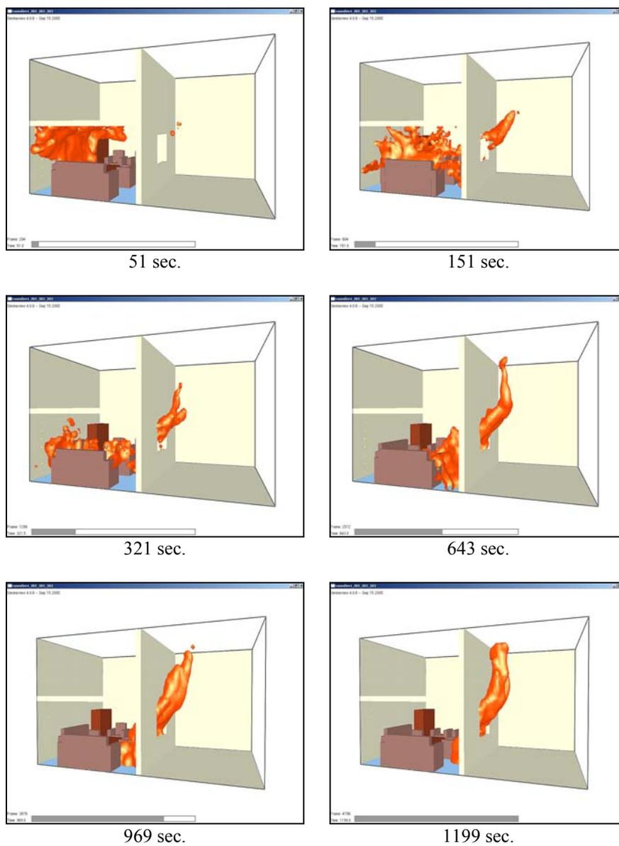
Fig. 2 Review of Fire Development from 51 to 1200 seconds since Ignition
