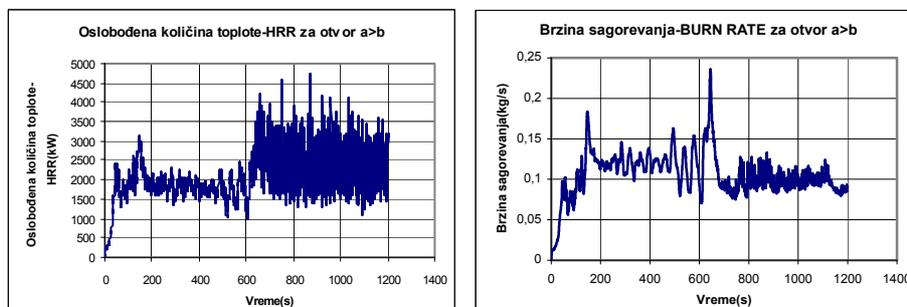
Fig. 4 Heat Release Rate and Burning Rate for Room with Opening 1.6 x 1.2 m
