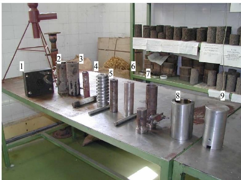
Fig. 5.4. Tools for dry and wet briquetting procedures used in Combustion laboratory at the Faculty of Occupational Safety in Nis (design D.Mitic, photo "Inkoplan", Nis), from the left to the right:
