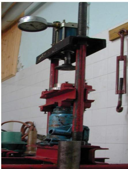
Fig. 5.8. Press for briquettes pressure resistance test (photo: "Inkoplan", Nis)
