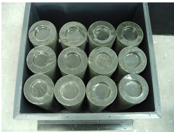
Fig. 4 Adsorption filter in the form of a cluster group
