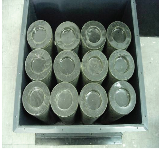
Fig. 5. Adsorber in the purifier module in the form of a cluster group [2]
