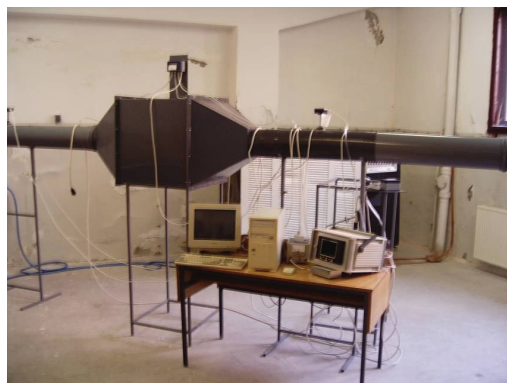
Fig. 1. Module of integrated air purifier and data acquisition system [2]
