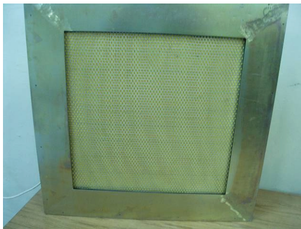
Fig. 3. Filter 109.122.73/20A, view of the rear side reinforced by perforated foil [2]
