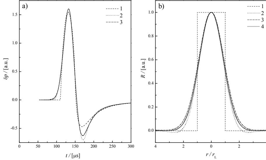
Fig. 1. A numerical simulation of the method for simultaneous determination of the laser beam profile and  $\tau_{v,T}$ . The simulated profile is Gaussian. The starting profile in simulation is a top-hat. a) Photoacoustic signals. b) The laser beam profiles. The solid lines depict real profile and photoacoustic signal.
