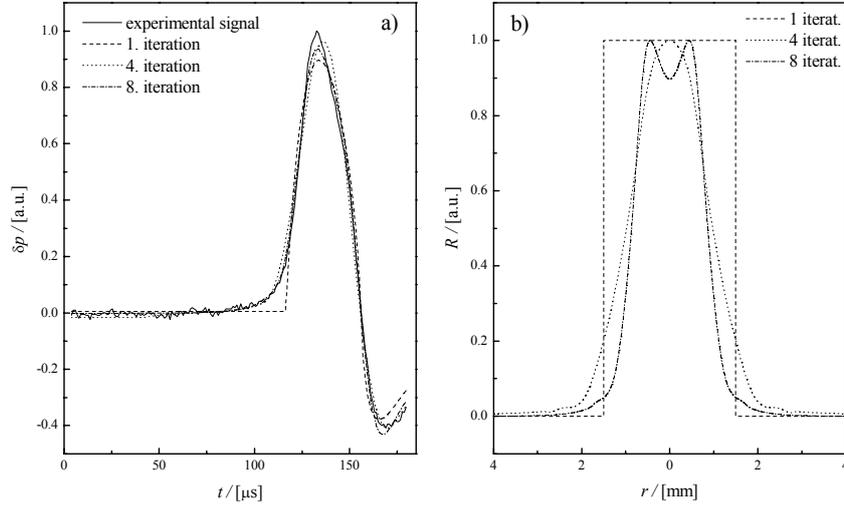
Fig. 2. An experimental example for determination of the laser beam profile and  $\tau_{v-T}$ . The experimental signal is obtained in SF<sub>6</sub>-Ar gas mixture. The starting profile in calculation is top-hat. a) The experimental photoacoustic signal (solid line) and obtained theoretical signals. b) Obtained laser beam profiles.
