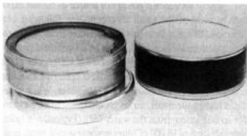
Fig. 3. Photographs of charcoal canisters made according to EPA standards
