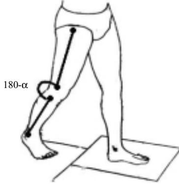
Fig. 3. Definition of the knee angle ( $\alpha$ ). The knee angle is defined as the angle between a spatial vector joining the lateral malleolus to the fibula head and a spatial vector joining the lateral femoral epicondyle to the greater trochanter.
