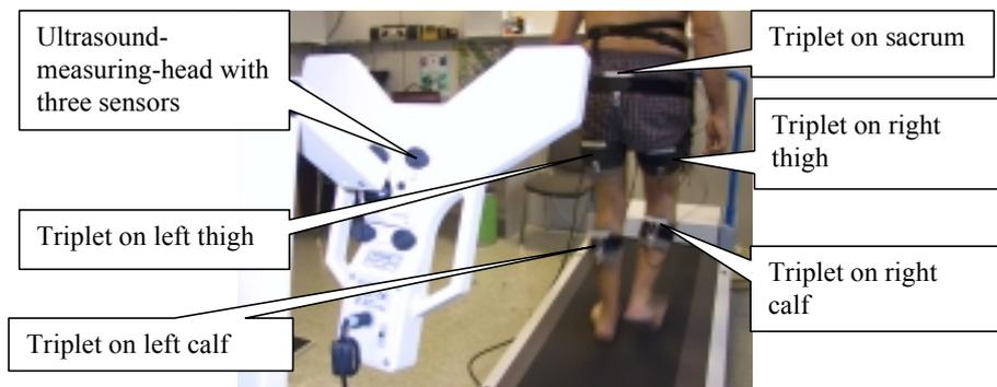
Fig.1. The arrangement of the measurement
