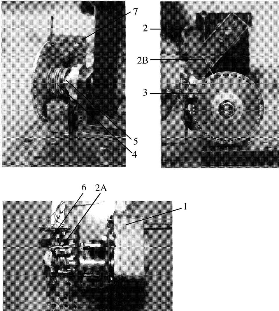
Fig. 3. The device for displacement measurements of the element driven by a helical torsional spring.
