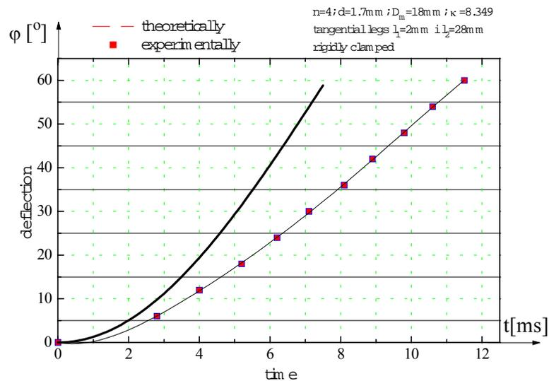
Fig. 6. Time dependence of the angular motion for an element driven by a helical torsion spring.
