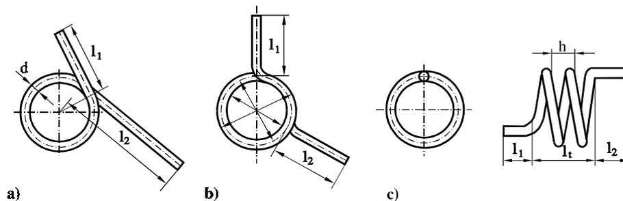
Fig. 2. Three different types of helical torsional springs.
