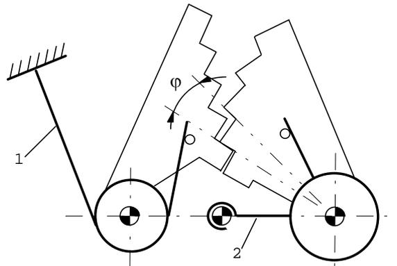
Fig. 1. Helical torsional springs as driving elements.
