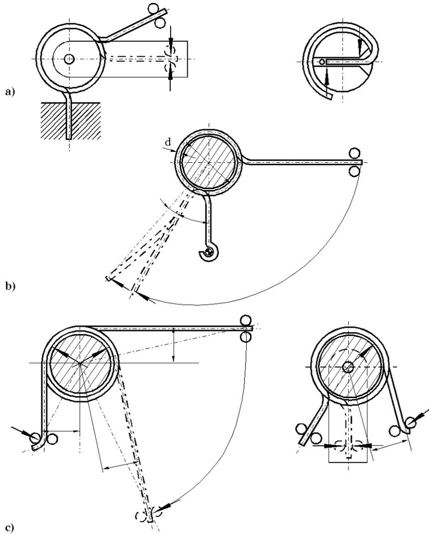
Fig. 4. A constructive solution of the different types of connection between the fixed spring end and the frame.
