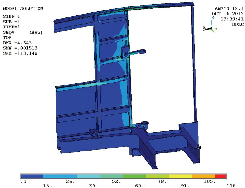
**Fig. 2** Stresses in coach structure near door under maximum lift service load
