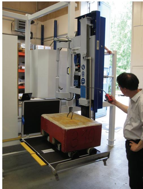
**Fig. 4** Lift tests in mock-up
