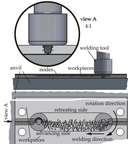
**Fig. 5** Scheme of nodes and their positions after numerical calculations
