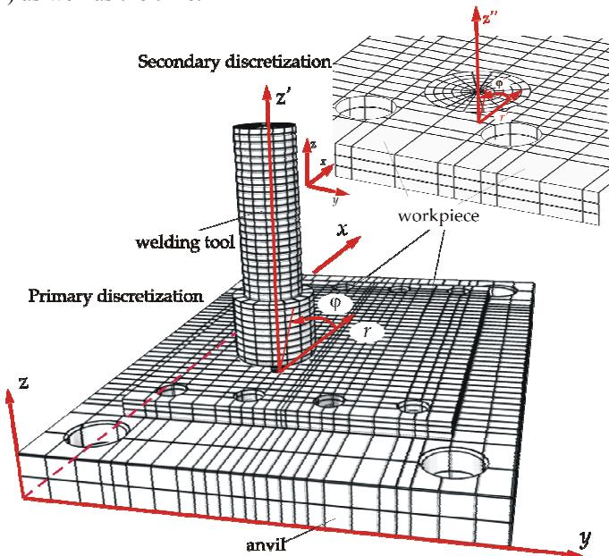
**Fig. 3** Primary and secondary discretization of the space
