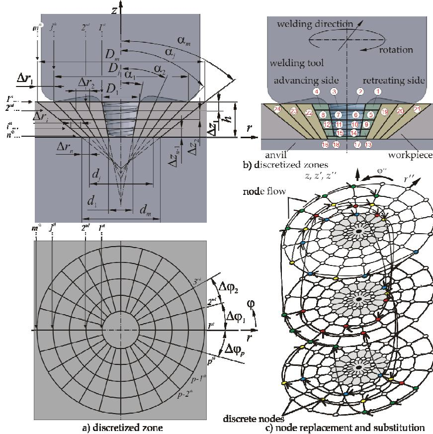
**Fig. 4** a) Secondary discretized space, b) Zones of material deposition,
