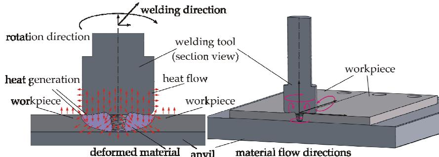
**Fig. 1** FSW scheme: heat generation, heat flow and material flow directions [8]
