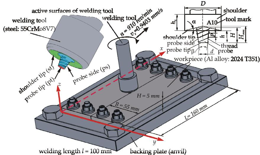
**Fig. 2** Details of numerical simulation and experimental investigation
