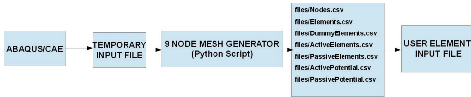
Fig. 3 Input and output of the 9-node mesh generator
