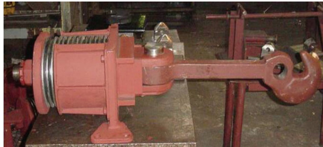
Fig. 1 The draw gear assembly filled with the rubber-metal spring
