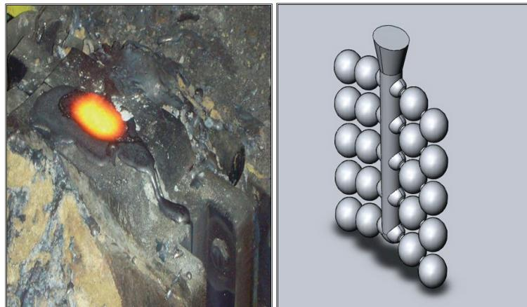
**Fig. 3** a) Pouring of cast iron into the tool; b) "balls in a cluster" after being taken out of the tools
