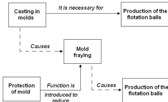
**Fig. 6** Graphical display of useful and harmful functions of the system
