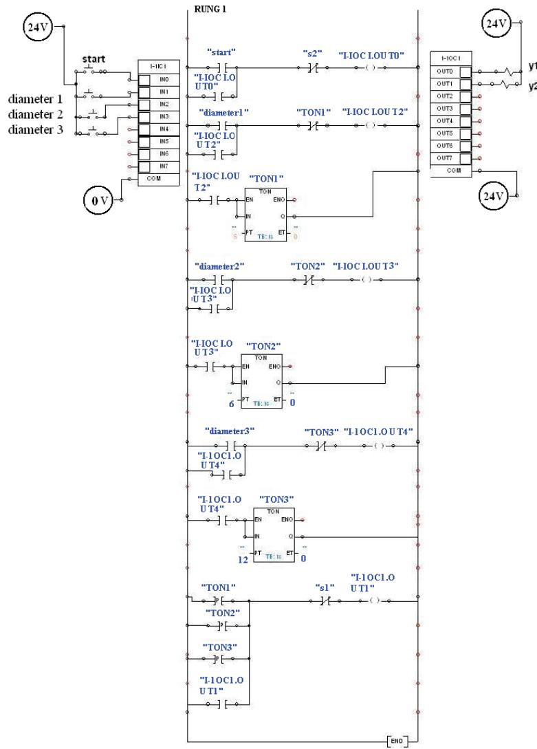
**Fig. 10** Managing the process by Ladder diagram
