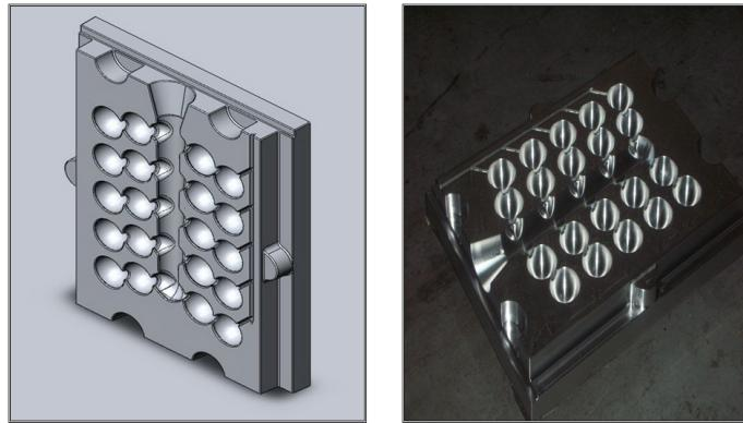
**Fig. 2** a) Drawing of the tool for balls casting;
