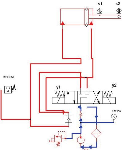
**Fig. 9** Hydraulic scheme - closed tool
