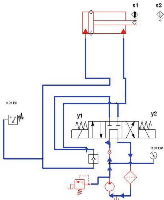
**Fig. 8** Hydraulic scheme - opened tool
