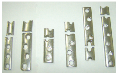
Fig. 1 Six investigated plates with cut parts for SEM analysis of failure surface
