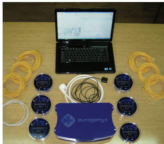
Fig. 1 The developed portable measurement and data acquisition system for analyzing dynamic characteristics of vehicles
