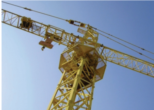
Fig. 1 Truss supporting structure: Photo of Tower crane Potain 744e
