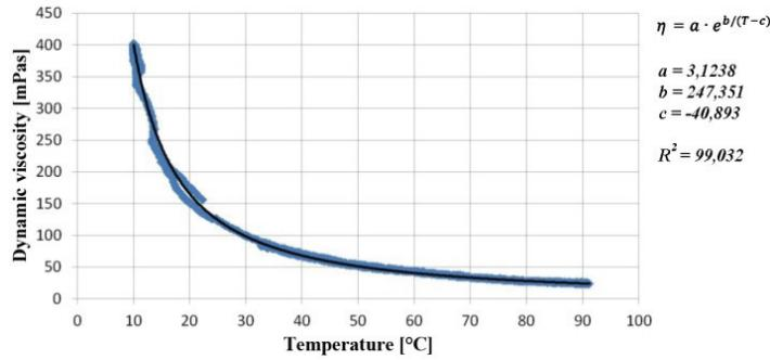
**Fig. 3.** Experimental viscosity-temperature calibration curve
