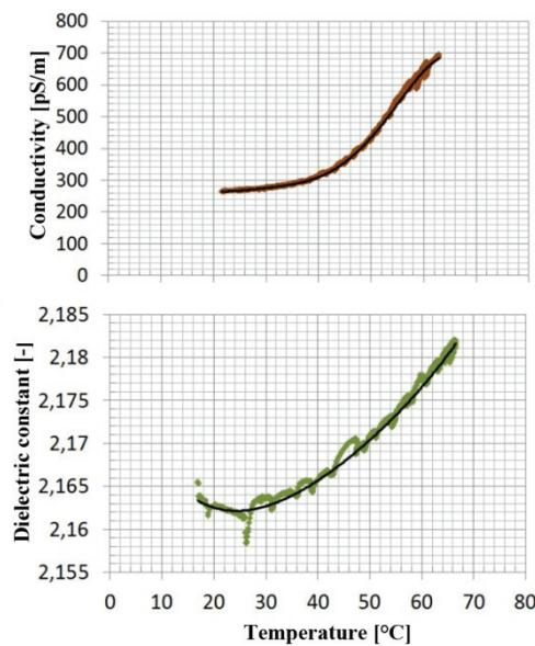
**Fig. 5.** Temperature dependency of electrical conductivity and dielectric constant for mineral hydraulic oil
