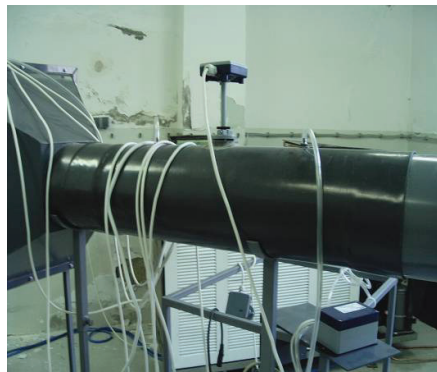
Fig. 4. Secondary transport duct with temperature and relative humidity transmitter
