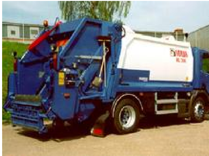
Fig. 1 "Norba" utility vehicle for communal waste transport
