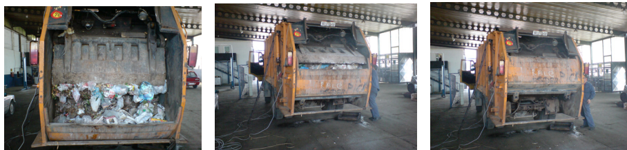
Fig. 4 The waste compression working cycle on a "Norba" system vehicle
