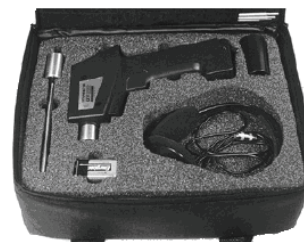
Fig. 6 The ultrasonic detector kit for Ultraprobe 100
