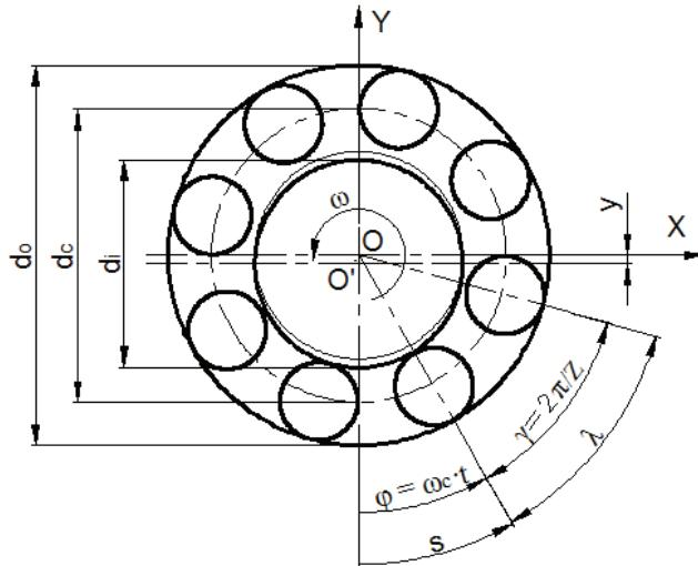
Fig. 1 Schematic Presentation of Rolling Bearing Kinematics
