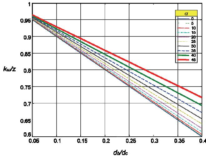
Fig. 4 Dependence of  $k_{\omega}/z$  Ratio on the Ratio of Rolling Bodies Diameter and Intermediate Diameter of the Cage ( $d_b/d_c$ ) for Various Values of Contact Angle  $\alpha$
