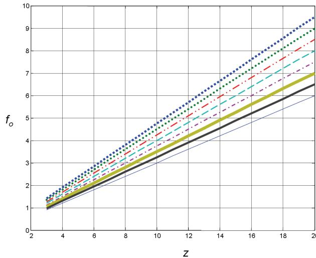
Fig 3 Dependence of Factor  $k_\omega$  on the Number of Rolling Bodies for Various Values of Diameter of Rolling Bodies and Intermediate Diameter of the Cage Ratio ( $d_b/d_c$ )
