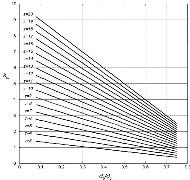
Fig 2 Factor  $k_\omega$  Dependence on Ratio  $d_b/d_c$  and Rolling Bodies Number ( $z$ ) for Single Breasted Round Bearing with Radial Contact
