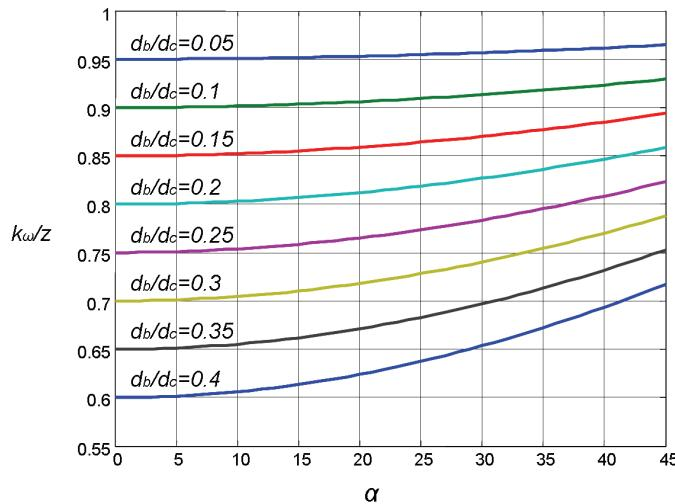
Fig. 6 Dependence of  $k_\omega/z$  Ratio on Contact Angle  $\alpha$  for Various Values of Rolling Bodies Diameter and Intermediate Diameter of the Cage ( $d_b/d_c$ )
