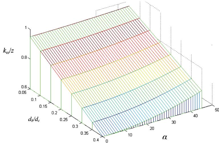
Fig. 5 Three Dimensional Dependence of  $k_{\omega}/z$  Ratio on the Ratio of Rolling Bodies Diameter and Intermediate Diameter of the Cage ( $d_b/d_c$ ) and Contact Angle  $\alpha$
