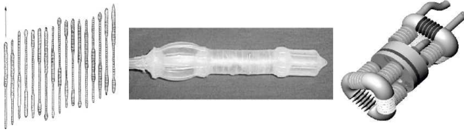
Fig. 1. Phases of locomotion of inchworm, a fiber reinforced 3-chamber hydraulic device with inchworm-like locomotion form
