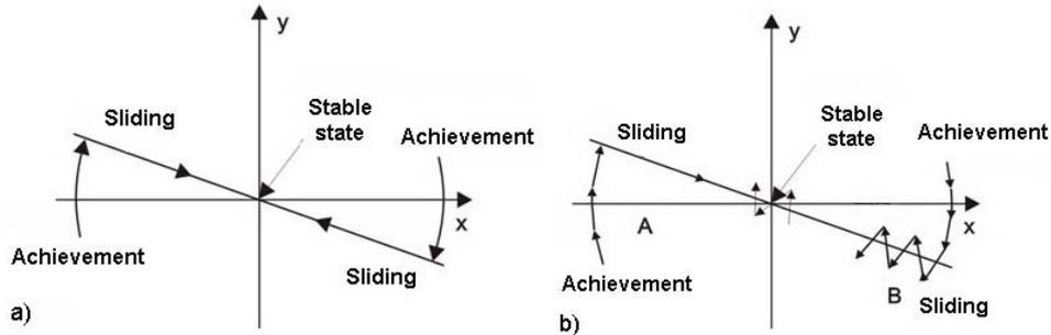
Fig. 2. Variable Structure System Trajectories: a) Analog, b) Digital
