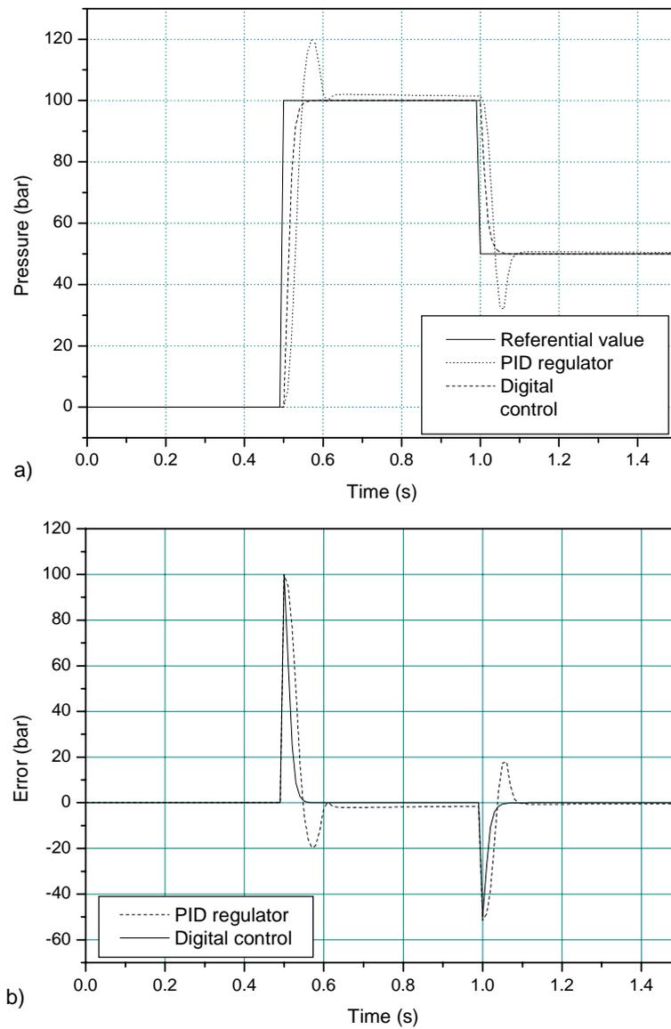
Fig. 3. Simulation Results: a) Tracking Bouncing Signal of Referential Pressure, b) Error
