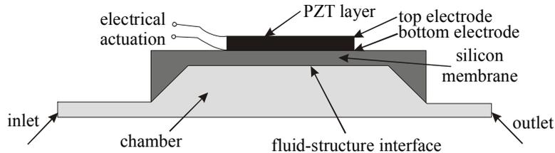
Fig. 1. A Cross-sectional View of Piezoelectric Micropump
