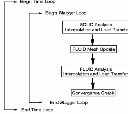
Fig. 2. Fluid-solid Sequential Coupling Algorithm for the Time and Stagger Loops
