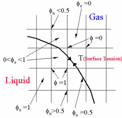
Fig. 3. Representation of the VOF Method with the Free Contact Surface of Immiscible Fluids
