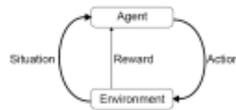
Fig. 9. Interaction between RL-system and the process
