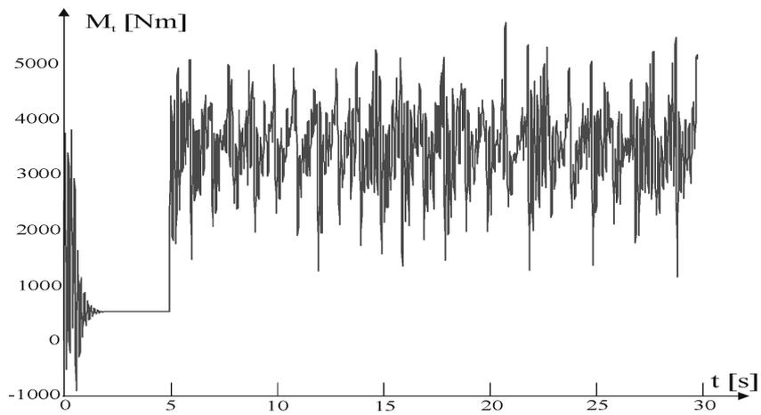
Fig. 6. Change of the twisting moment of the power gear's input shaft
