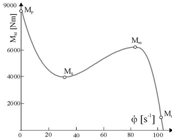
Fig. 2. Curve of starting the motor
