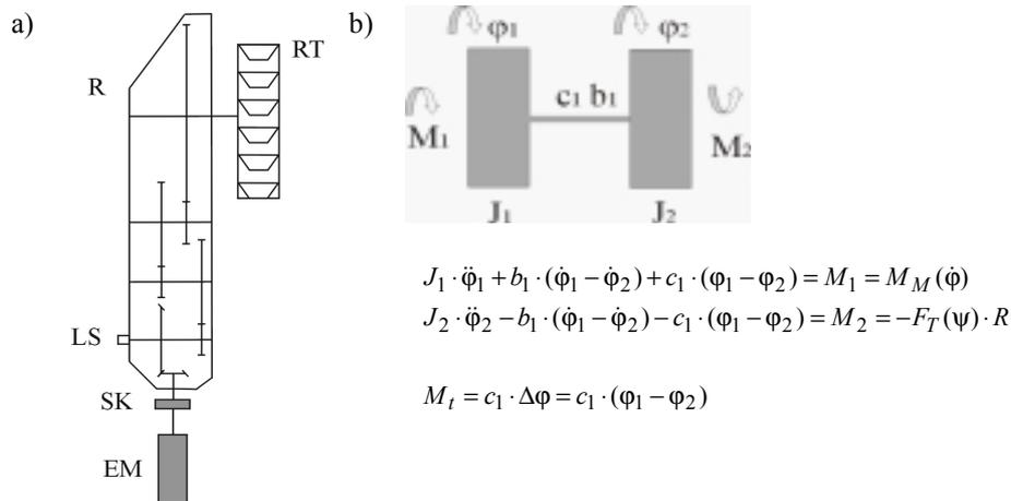
Fig. 1. a) Scheme of the driving system of the boogie-wheel of bucket wheel excavator SRs 470.20.3 LAUHAMER
