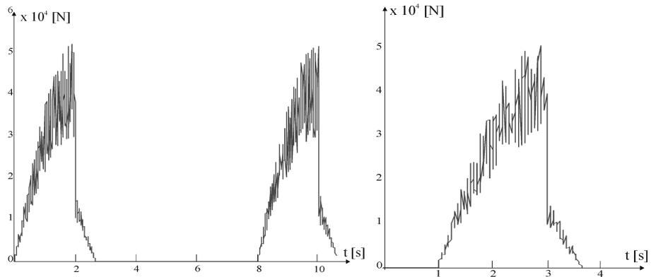
Fig. 4. Change of resistance to digging: a) of the first spoon b) of the second spoon
