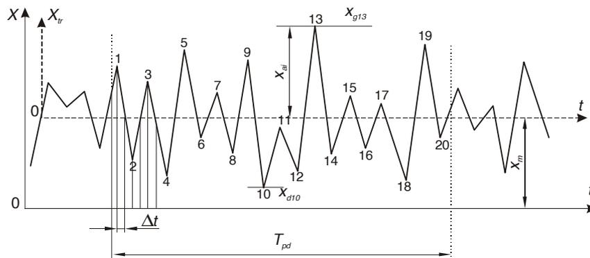
Fig. 3. Accidental function discretization
