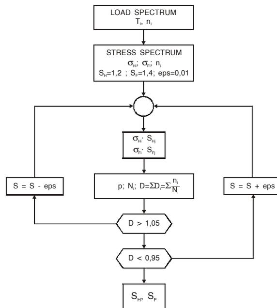
Fig. 7. The algorithm of the calculation factor of safety from tooth breakage and factor of safety from pitting
