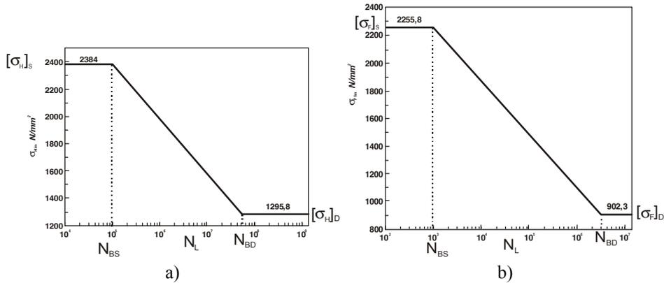
Fig. 6. Damage lines for damage statistical probability of 10%
