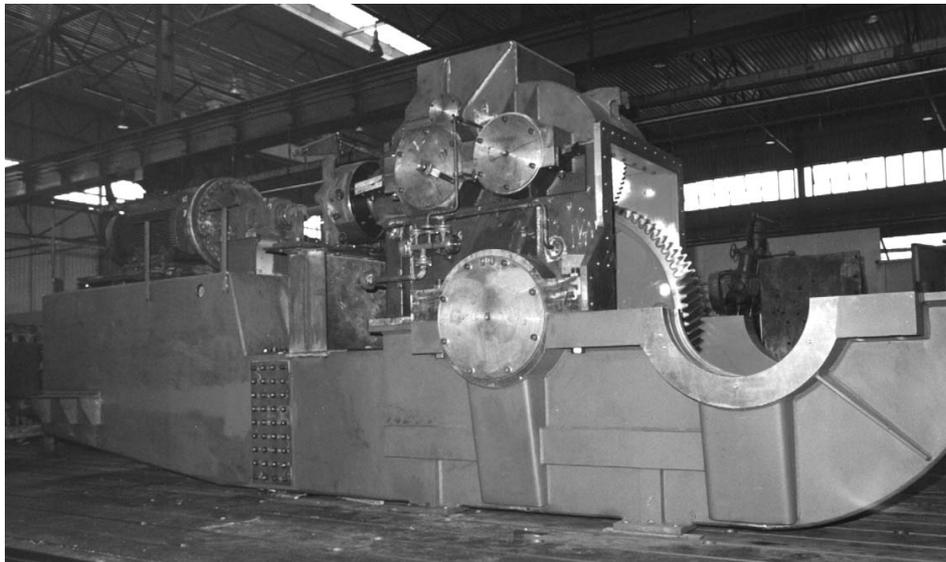
Fig. 2. Gear transmission of the bucket wheel excavator working wheel
