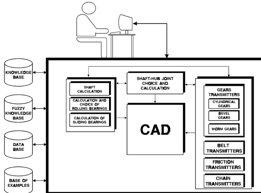
Fig. 4. Architecture of the program system for designing of power transmission
