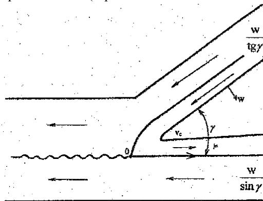
Fig. 3. Scheme of flow realized near the collision zone, coupled with the contact point, in regime subsonic oblique collision
