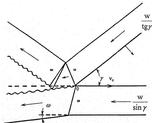
Fig. 4. Scheme of flow realized near the collision zone in regime of supersonic oblique collision with attached shock waves
