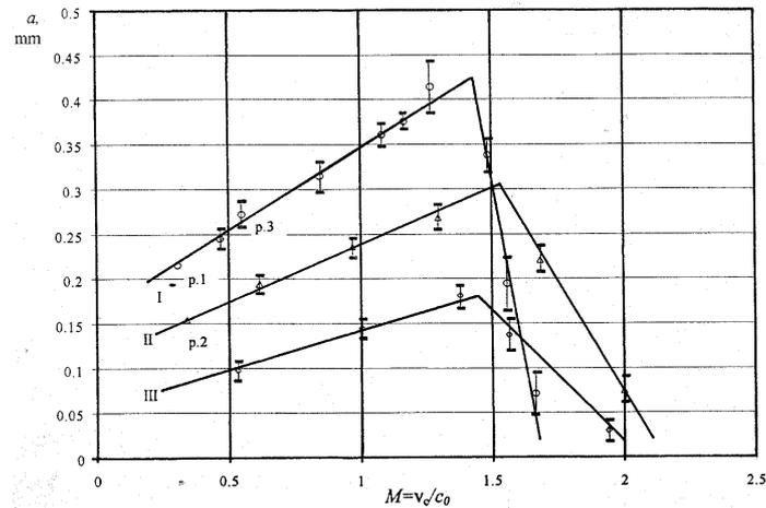
Fig. 2. Amplitude of perturbations on contact boundaries between metals layers versus Mach number: I - AlMgZn alloy - AlMgZn alloy; II - Copper - copper; III - Steel St.3 - steel St.3
