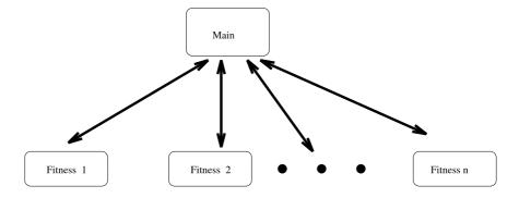
FIG. 2: Distributed implementation of the constructive genetic algorithm
