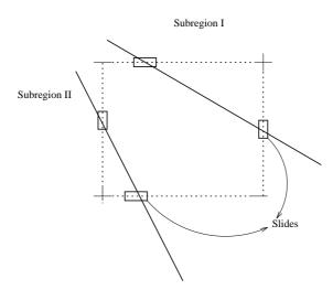
FIG. 1: The exclusive OR function realized by a neural network with two hidden units. The figure shows slides on the dotted lines between the points from the opposite classes. The slides can be in one of the k different positions on the dotted line.
