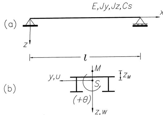
Fig. 1. Geometry, properties and sign convention of a simply supported beam with open monosymmetric cross section.
