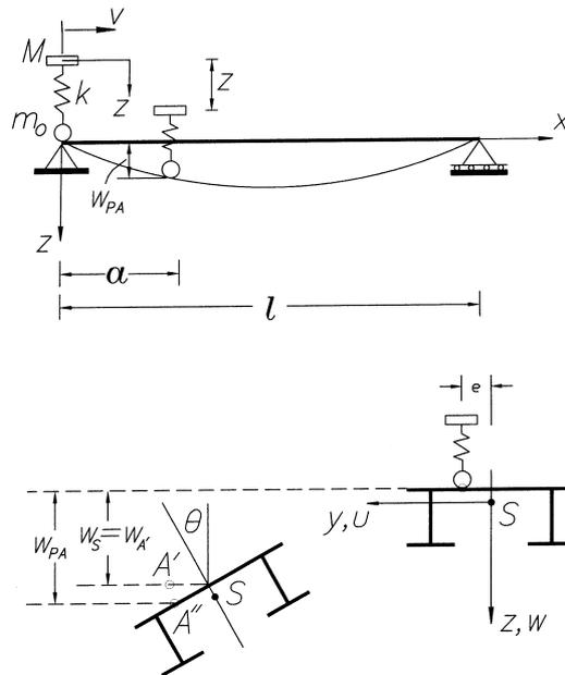
Fig. 3. The simply supported beam of Fig. 1, acted upon eccentrically by a two-mass vehicle model moving with constant velocity.
