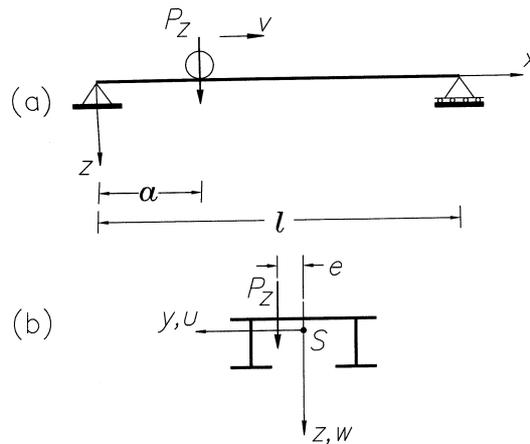
Fig. 2. The simply supported beam of Fig. 1, under the passage of a constant load moving with constant speed across the span eccentrically.
