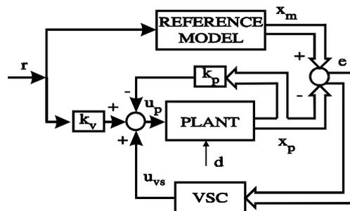
Fig. 1 Block-diagram of the first variable structure MRAC
