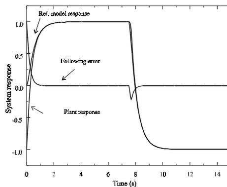
Fig. 3 Reference model and plant responses (first control algorithm)
