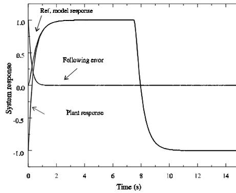
Fig. 4 Reference model and plant responses (second control algorithm)
