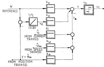
Fig. 3 Informational block diagram of the proposed sliding mode controller.
