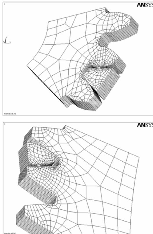
Fig. 2. 3D FEM model for gear pair in mesh
