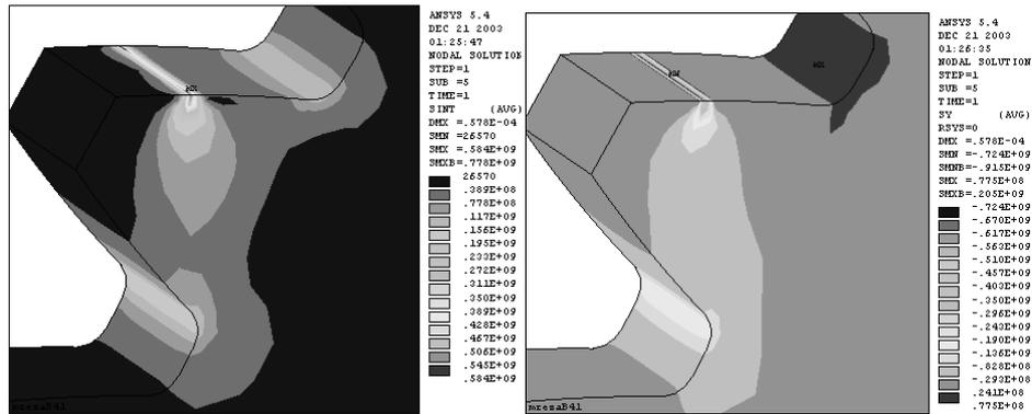
Fig. 5. Values of equivalent stress  $\sigma_{INT}$  and direct stress in y-direction  $\sigma_y$  for a wheel tooth
