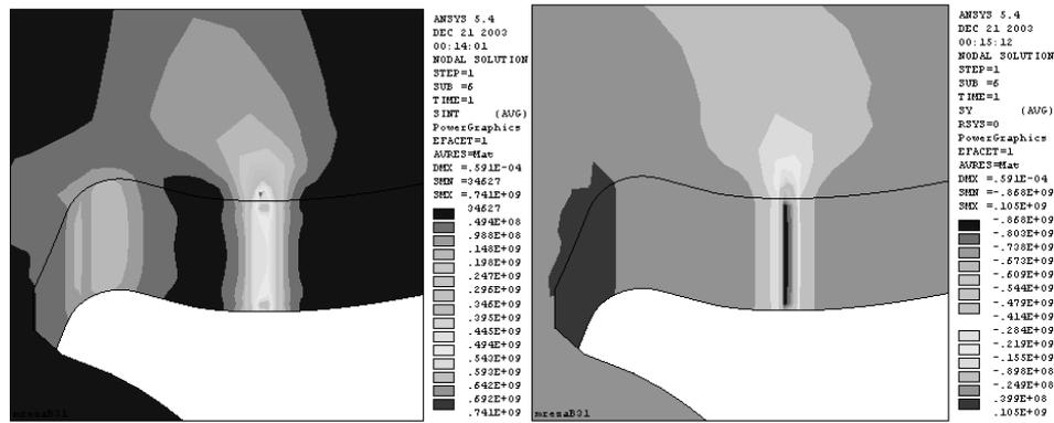
Fig. 4. Values of equivalent stress  $\sigma_{INT}$  and direct stress in y-direction  $\sigma_y$  for a pinion tooth
