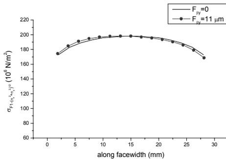
Fig. 13. Influence of mesh misalignemt on total root tooth stress variation along facewidth – pinion tooth
