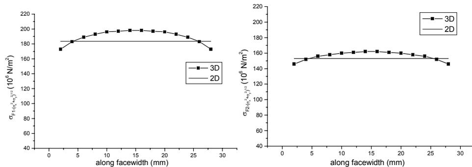
Fig. 9. Diagrams for monitoring of total tooth root stresses variation over facewidth – point B on path of contact (single meshed tooth pair period)
