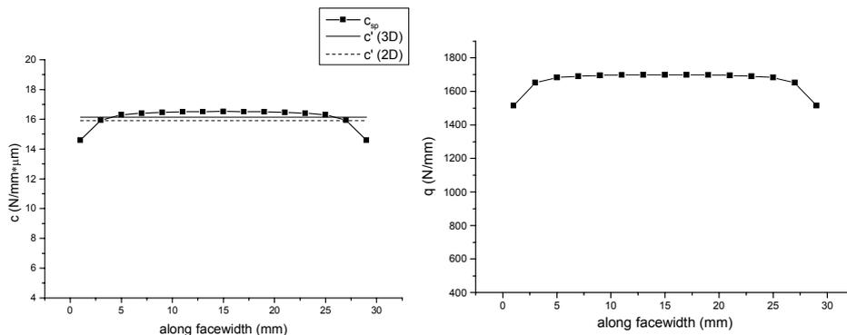
Fig. 7. Diagrams for monitoring of tooth stiffness and unit nominal load variation over facewidth – point B on path of contact (single meshed tooth pair period)
