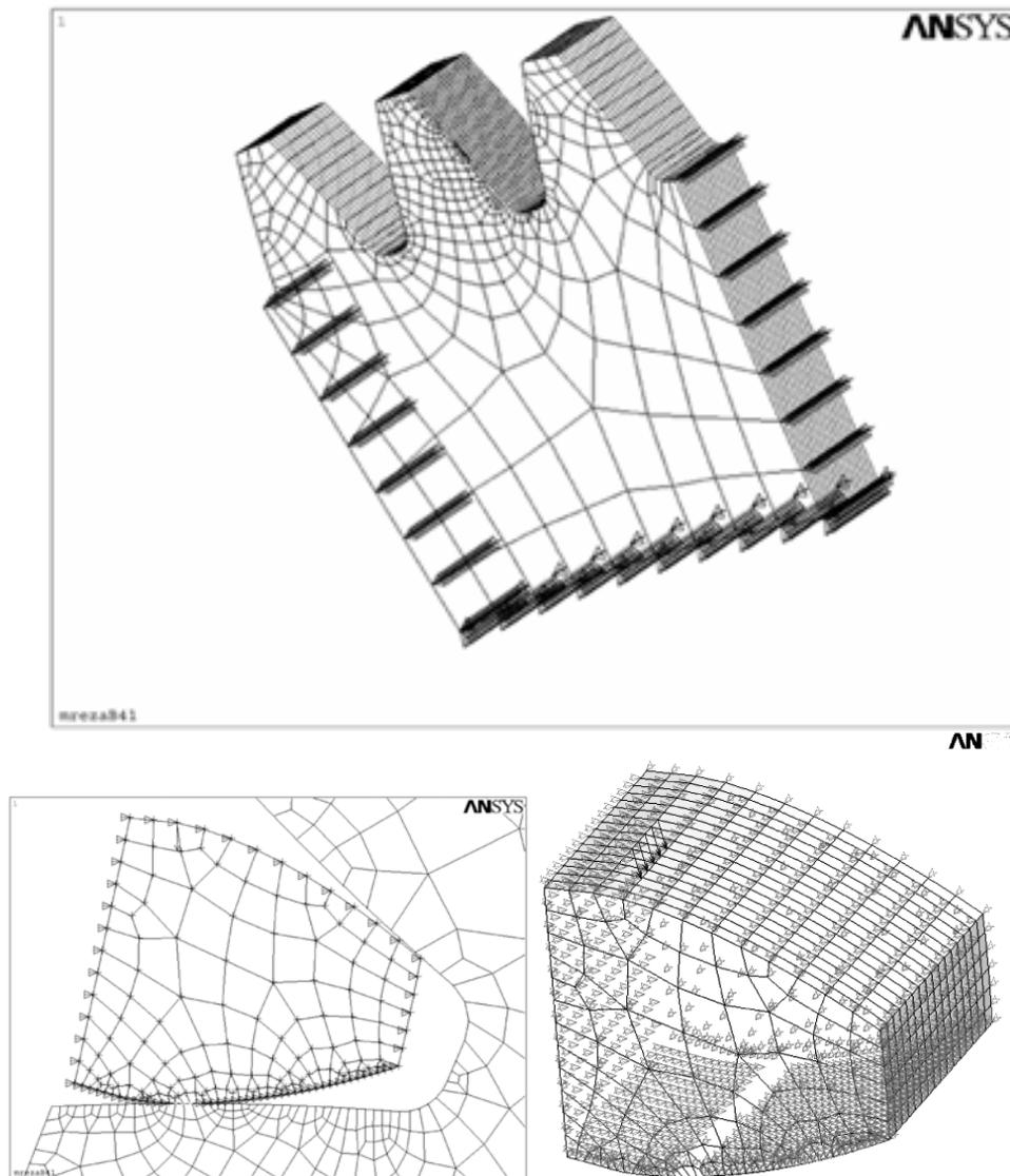
Fig. 3. Displacement constraints and external load application for 3D FEM wheel model
