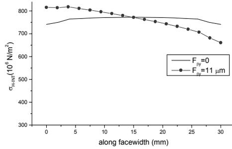
Fig. 12. Influence of mesh misalignemt on equivalent contact stress variation along facewidth
