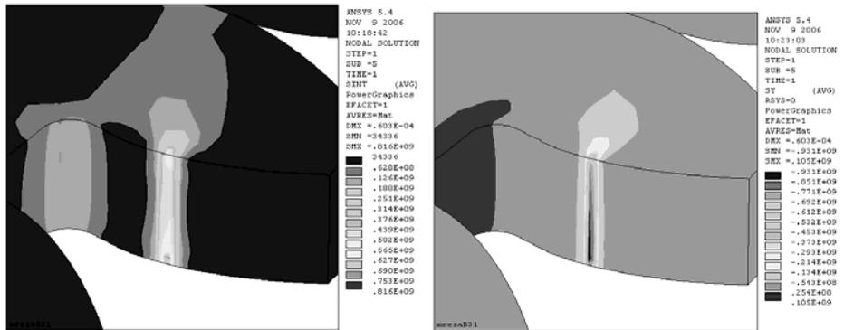
Fig. 10. Influence of mesh misalignemnt on equivalent stress  $\sigma_{INT}$  and direct stress in y-direction  $\sigma_y$  – pinion tooth
