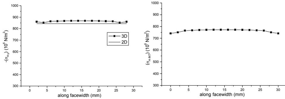
Fig. 8. Diagrams for monitoring of contact stress variation over facewidth – point B on path of contact (single meshed tooth pair period)
