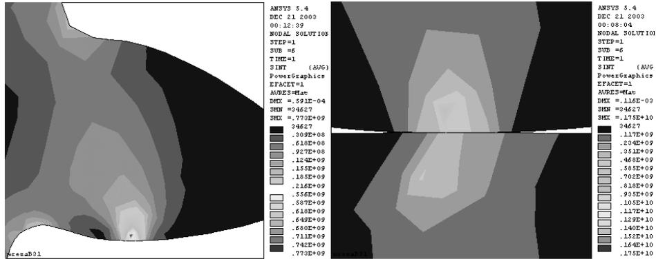
Fig. 6. Values of equivalent stress  $\sigma_{INT}$  for a pinion tooth in different cross sections along gear facewidth
