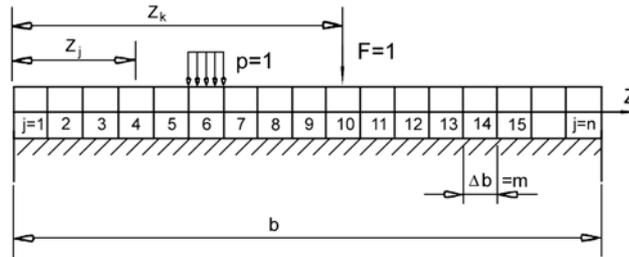
Fig. 1. Partition of tooth pair contact pattern on finale number of equal segments
