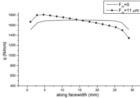
Fig. 11. Influence of mesh misalignemt on unit nominal load variation along facewidth
