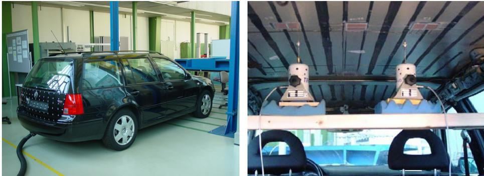
Fig. 1. a) VW test car "Bora"; b) passenger compartment and inner surface of the car roof with attached piezoelectric actuators/sensors and exciting shakers
