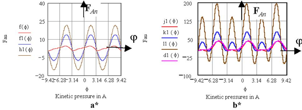
Fig. 3. a\* and b\* Graphical presentation of kinetic bearing pressures  $F_A$  for different values of system parameters: the eccentricity coefficient  $v = \frac{e}{r}$  and the angle  $\beta$ .
