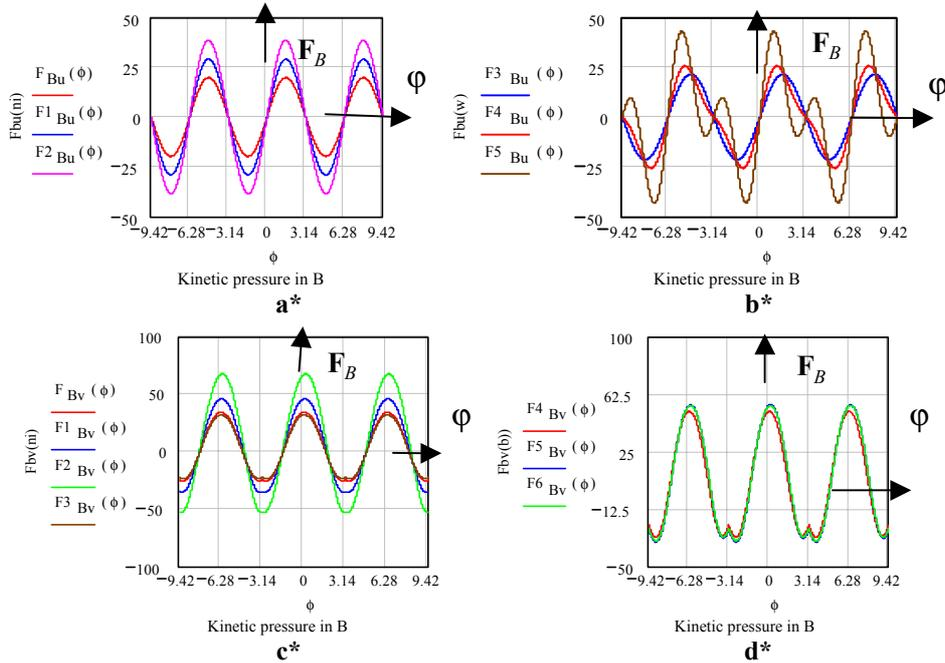
Fig. 7. a\*, b\*, c\* and d\* Graphical presentation of kinetic bearing pressures  $F_B$  for different values of system parameters: the eccentricity coefficient  $\nu = \frac{e}{r}$  and the angle  $\beta$ .
