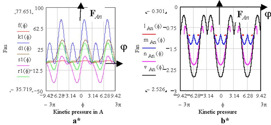
Fig. 6. a\* and b\* Graphical presentation of kinetic bearing pressures  $F_A$  for different values of system parameters: the eccentricity coefficient  $\nu = \frac{e}{r}$  and the angle  $\beta$ .
