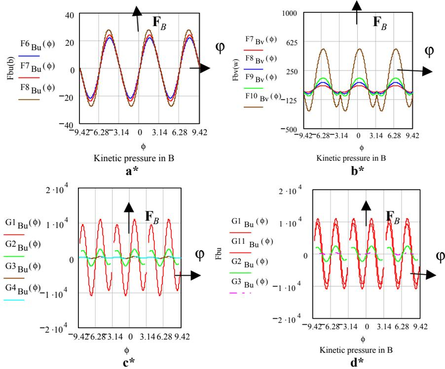
Fig. 8. a\*, b\*, c\* and d\* Graphical presentation of kinetic bearing pressures  $F_B$  for different values of system parameters: the eccentricity coefficient  $\nu = \frac{e}{r}$  and the angle  $\beta$ .
