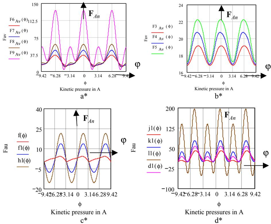
Fig. 5. a\*, b\*, c\* and d\* Graphical presentation of kinetic bearing pressures  $F_A$  for different values of system parameters: the eccentricity coefficient  $\nu = \frac{e}{r}$  and the angle  $\beta$ .
