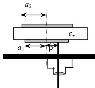
Fig. 1. Coax-fed inverted microstrip stacked patch resonator
