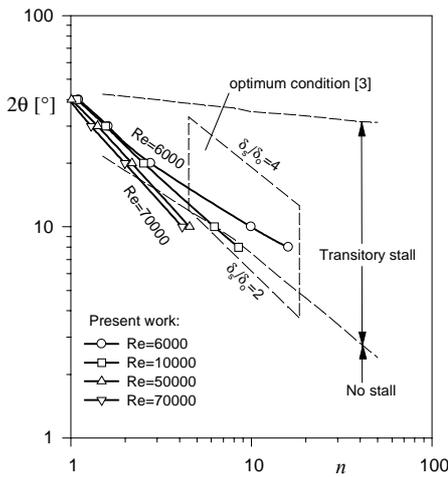
Fig. 4. Comparison of our results and the optimal regime flow in plane diffuser [3].
