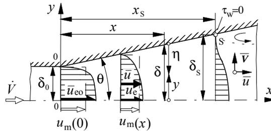
Fig. 1. Flow through a diffuser
