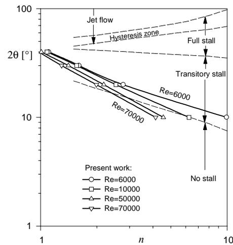
Fig. 3. Dependence of the separation point on the parameters:  $Re$ ,  $\theta$  and  $n$ . Dash lines correspond a Kline's diagram and full lines correspond at our results.
