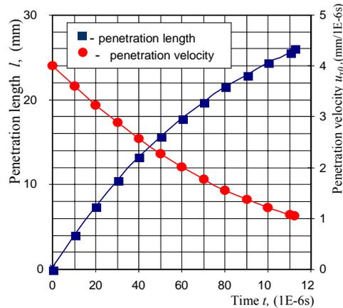
Fig. 4. The jet penetration length and velocity depending on time
