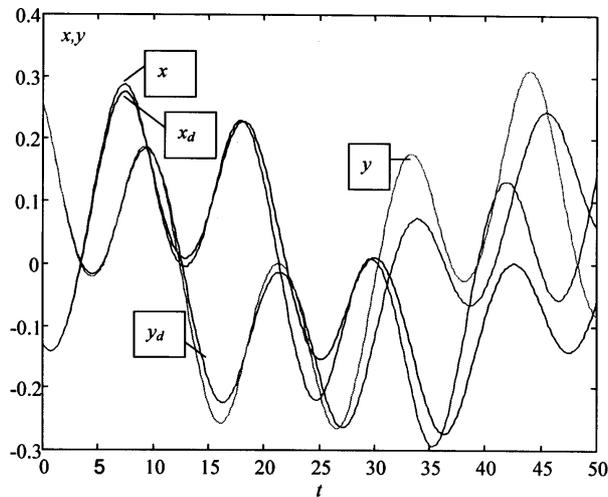
Fig. 2. The time history diagrams of rotor center  $x-t$  and  $y-t$  for the case without damping and  $x_d-t$  and  $y_d-t$  for the case with damping
