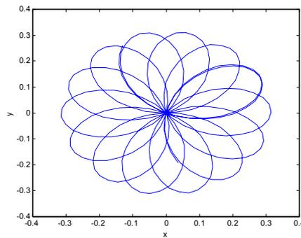
Fig.1. The orbital motion of the rotor center
