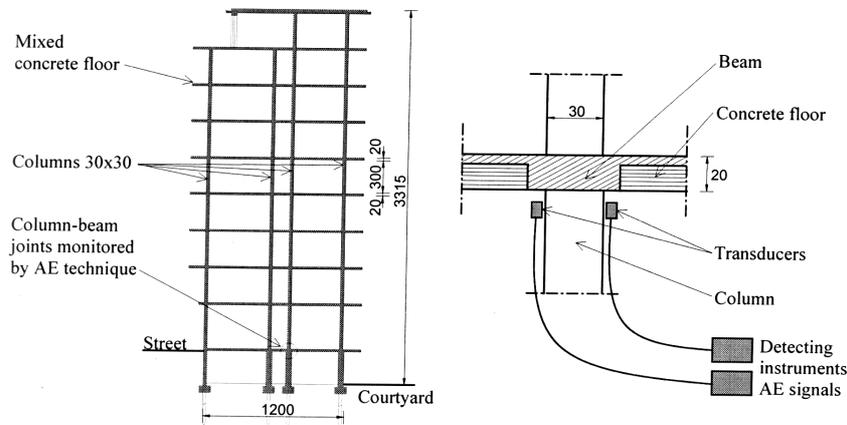
Fig. 2. Building in Moncalieri. Structural section of the building and location of transducers on column-beam joints
