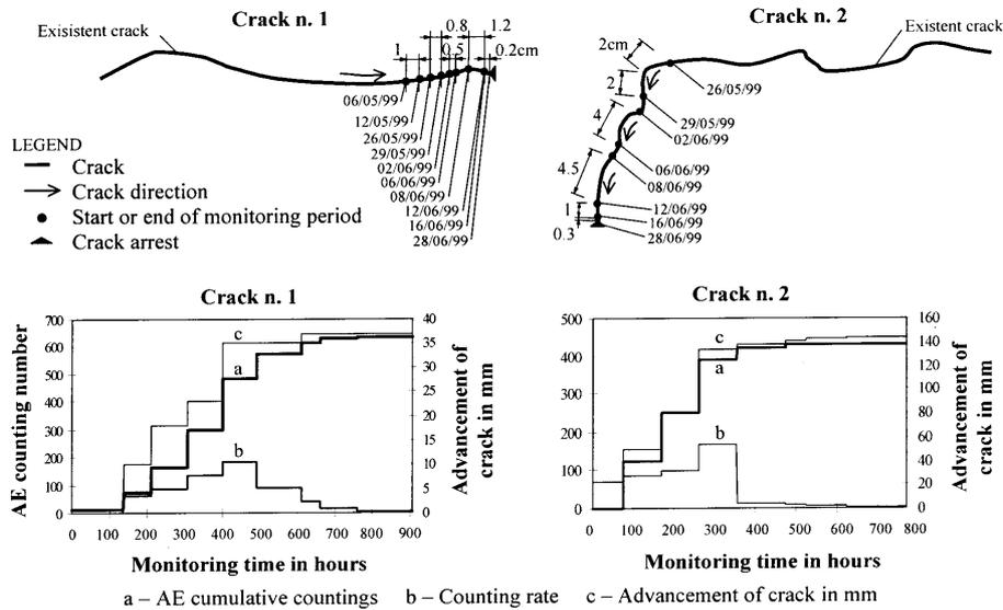
Fig. 7. Crack n. 1 and 2. Development and AE monitoring results
