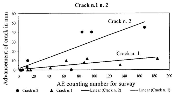
Fig. 8. Diagrams of correlation between the number of AE events and the crack advancement
