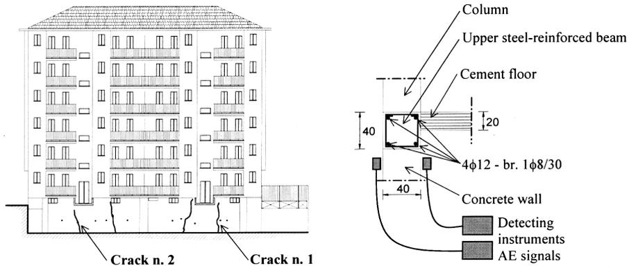
Fig. 4. Building in Cascine Vica. Cracking framework and location of transducers on the concrete wall
