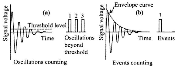
Fig. 1. Detected signals by AE technique
