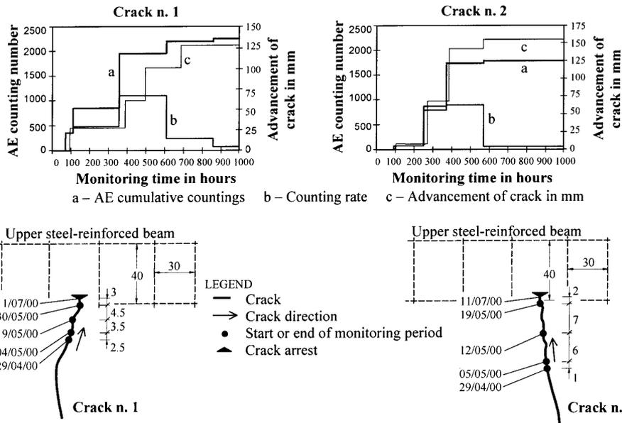
Fig. 5. Results of monitoring with the AE technique
